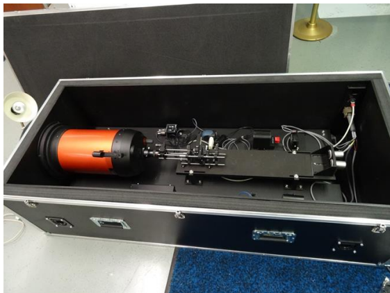
Figure 34: Box containing the telescope, the optical elements and the two fiber collimators on the right hand side. The box is controlled in temperature and located outside in harsh conditions (wind, temperature). The two optical fibers transmit the signal to a spectrograph and a CCD camera located 50 meters away inside the observatory in Skibotn.
