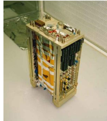
Figure 36: The DIARAD/VIRGO instrument built by Verhaert NV in collaboration with the Royal Meteorological Institute of Belgium (RMIB).
